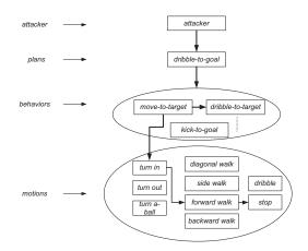
Fig. 2. A sample instantiation of the *dribble-to-goal* plan.
