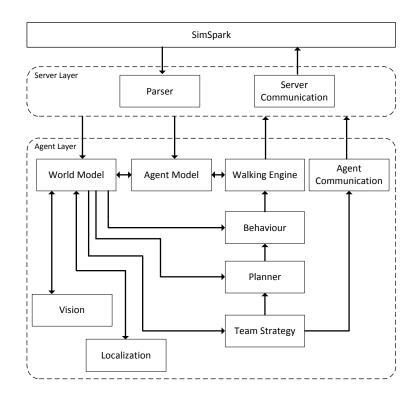
Fig. 1. Overall Software Architecture.
