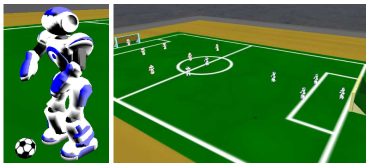
Figure 1. On the left is a screenshot of the Nao agent, and on the right a view of the soccer field during a 6 versus 6 game.
