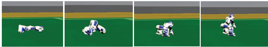
Fig. 6. Different phases of the stand up behavior
