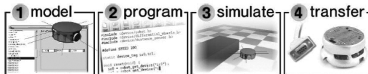
Fig. 2. Webots development cycle of robot simulation.
