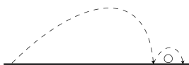
Fig. 3. Ball velocity is reduced after first bounce so the ball can be intercepted
